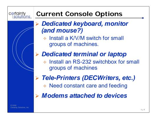
Dedicated monitors for each machine would be impractical. The cost for PC K/V/M ports are cheaper than serial consoles, but are more expensive for other platforms.
