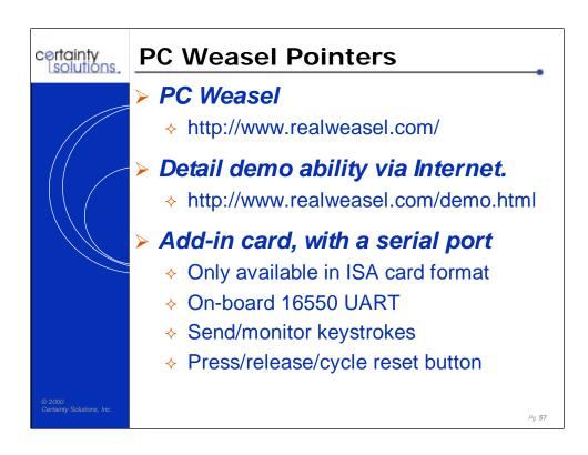
The devices appears to the computer to be a monochrome video adapter. The P.O.S.T. information that is sent to the video adapter interface is then sent to the serial port on the card.
