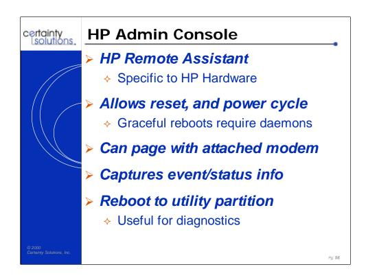
Some Netserver CPUs have some remote control capability built in. (HP/UX does have the ability to use a serial port as a console,) You can also add the control capability by installing an HP Remote Assistant management card, with connections to the motherboard for some control functions. You also need the NetServer Navigator CD to configure the system.
