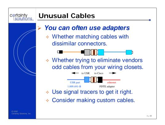
When connecting a DB-type connector to another DB-type connector, you can use adapters on each device, and a CAT-5 cable in between. (When you do this, the RJ-45 format must be the same for both adapters.) Then use the passive signal tracer to verify that the signals look correct on both ends.
