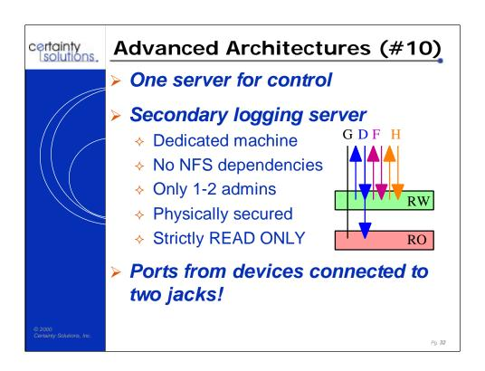
Legend: G = signal ground, D = tx and rx data, F = hardware flow control leads, and H = hardware handshaking leads.
