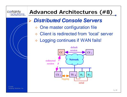
In the case of Conserver, you can indicate in the configuration file which of a number of distributed conserver hosts is maintaining the logs for any particular device, as well as indicating which remote terminal server is directly connected to the device.
