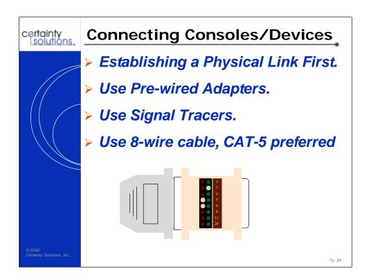
Once your terminal server is connected, your next task is to connect various serial consoles to the terminal server ports.
