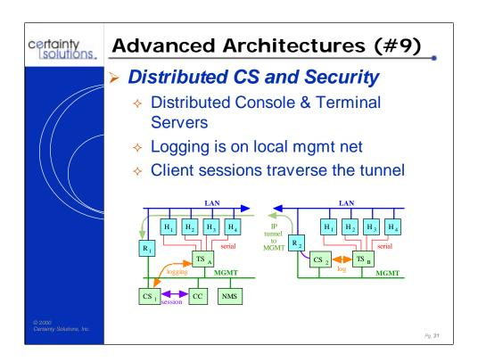
We can extend the idea of distributed console server hosts in our earlier security models. In this case, all of the logging traffic is kept on the remote management network, as peer-to-peer traffic, and only the client sessions from other sites is carried over the tunnel.
