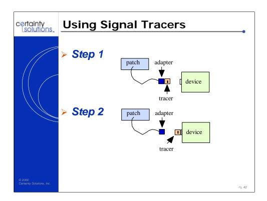
When you use pre-wired adapters, the first step is to make sure you are using an adapter with the RJ-45 connector wired for your terminal server. (This may mean that you have a pair of adapters, DTE and DCE, with the appropriate connectors for your host...at this point, you should pick one to test with.)
