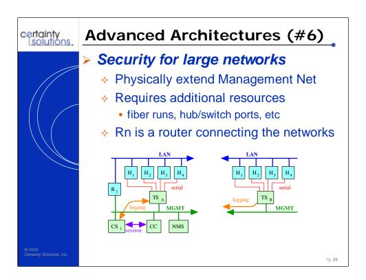
If you have a need to support multiple data centers, you may want to extend your management network to those other data centers. (Remember that serial lines have fairly limited distances, and it is easier to extend an ethernet network than to extend serial lines.)
