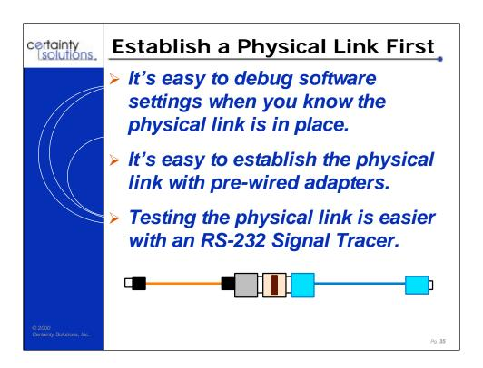
You could use an asynchronous serial protocol analyzer to determine whether your software settings are correct. Or, you could use a small, passive device to help you get the hardware signals in place.
