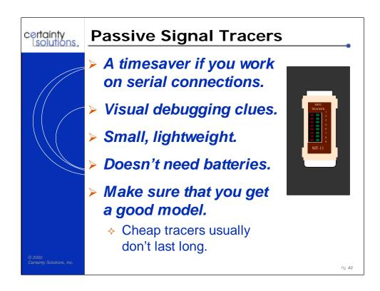
In my opinion, a passive signal tracer is more useful than a breakout box for most testing circumstances. I believe this because most cases do not require us to make special crossover cables, or jumper pins together, especially when you use pre-wired adapters that support all handshaking and flow control leads.
