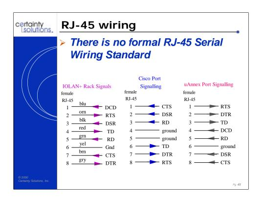
Receive Data (RD) is **usually** an input, but not always. (This confusion is prevalent between DTE and DCE devices, where the question is usually "Is RD a signal input, that I am receiving; or is it a signal that I output, sending data to the receiver of the DTE.?".)
